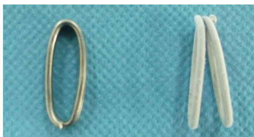
Figure 1. Nickel-titanium clip with two-way shape memory. Left: locked clip at room temperature. Right: open clip after cooling
